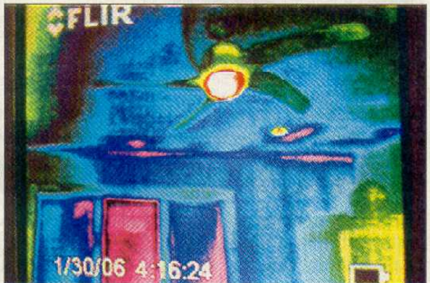
This is what the infrared camera sees: The darker colors indicate cold spots and the white indicates the hottest spots.
