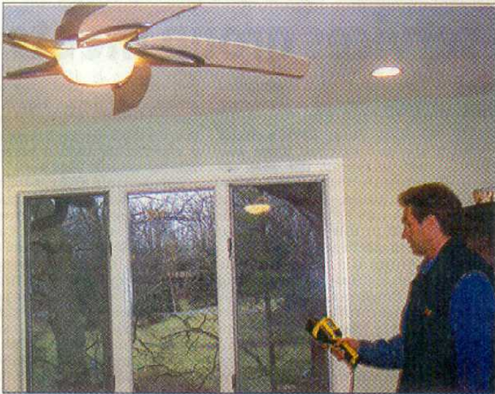
Jack Griffith, owner of Infrared Energy Analysis, uses an infrared camera to detect cold spots in the walls, ceiling and around the windows of a home.
